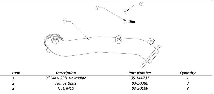
**aFe POWER recommends professional installation on this product.** Thoroughly inspect the aFe POWER downpipe to make sure there is no damage from shipping (if damage is noted, immediately contact aFe POWER customer service). Allow time for your vehicle to cool down prior to installation. When working on your vehicle proceed with caution. Wear protective safety equipment; eye goggles and gloves to ensure a safe installation.
